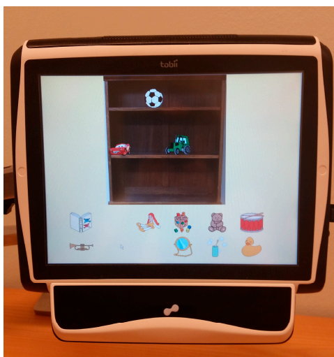
Figure 2. Example of a page with a play activity in the eye-gaze control technology. When fixating ones eye gaze on a toy, it moves to the shelf.
